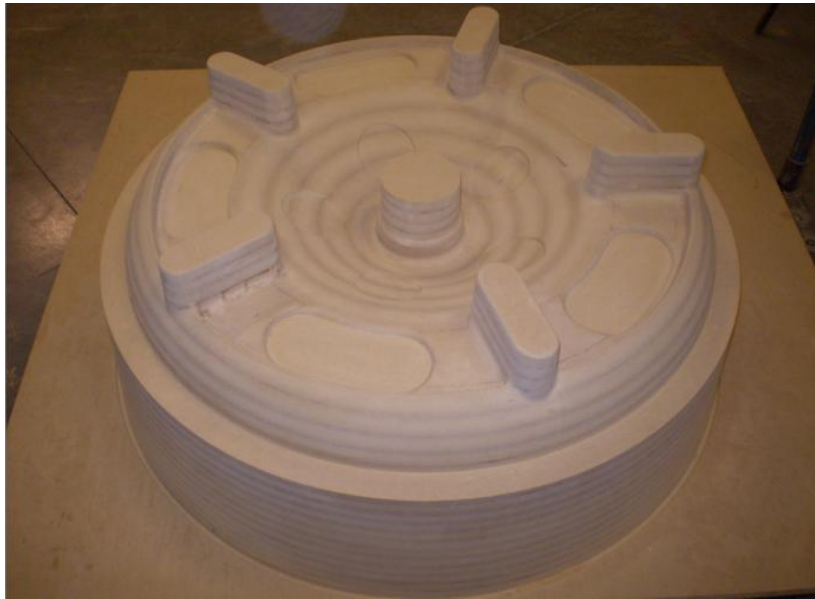
Figure 1.4- Pattern created from the Rapid Pattern Manufacturing process [Luo (2009)]
