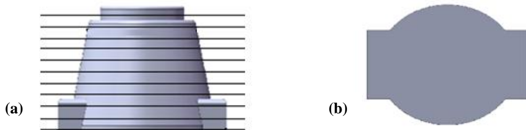
Figure 3.7- (a) Slicing of mold geometry (b) Union of all slices
